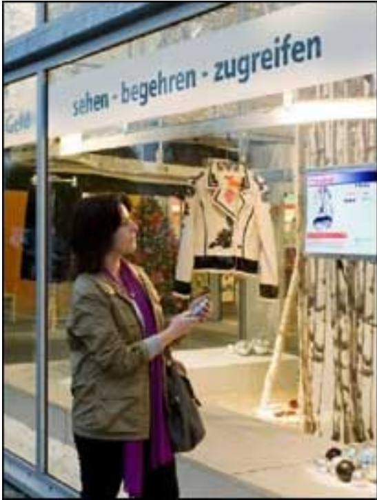
When a garment reaches the store window, an interrogator reads the item's RFID tag, prompting product information to appear on a computer screen.
