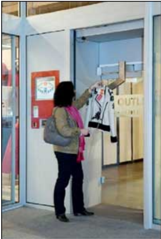
After a customer pays for an item, an RFID-enabled conveyor system delivers it directly to the purchaser.
